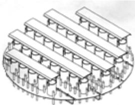
Pictured at the left is a typical liquid distributor designed to provide excellent water distribution over a wide turn down ratio. Note the multiple risers, orifices and drip tubes assuring gas and liquid separation, hence minimum pressure drop is .25" WC or less.
